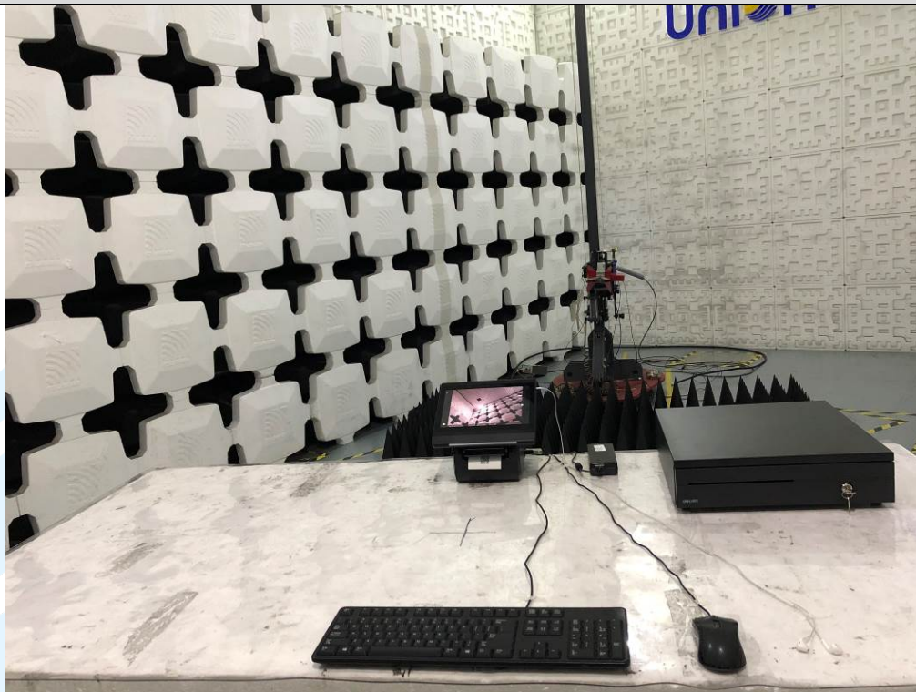
Radiated emission Test Setup-2 (Above 1 GHz) – Test Mode 1
