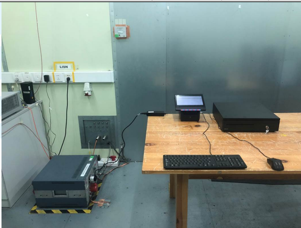
Conducted Emission Test Setup-3 – Test Mode 4 (Test Mode 2)
