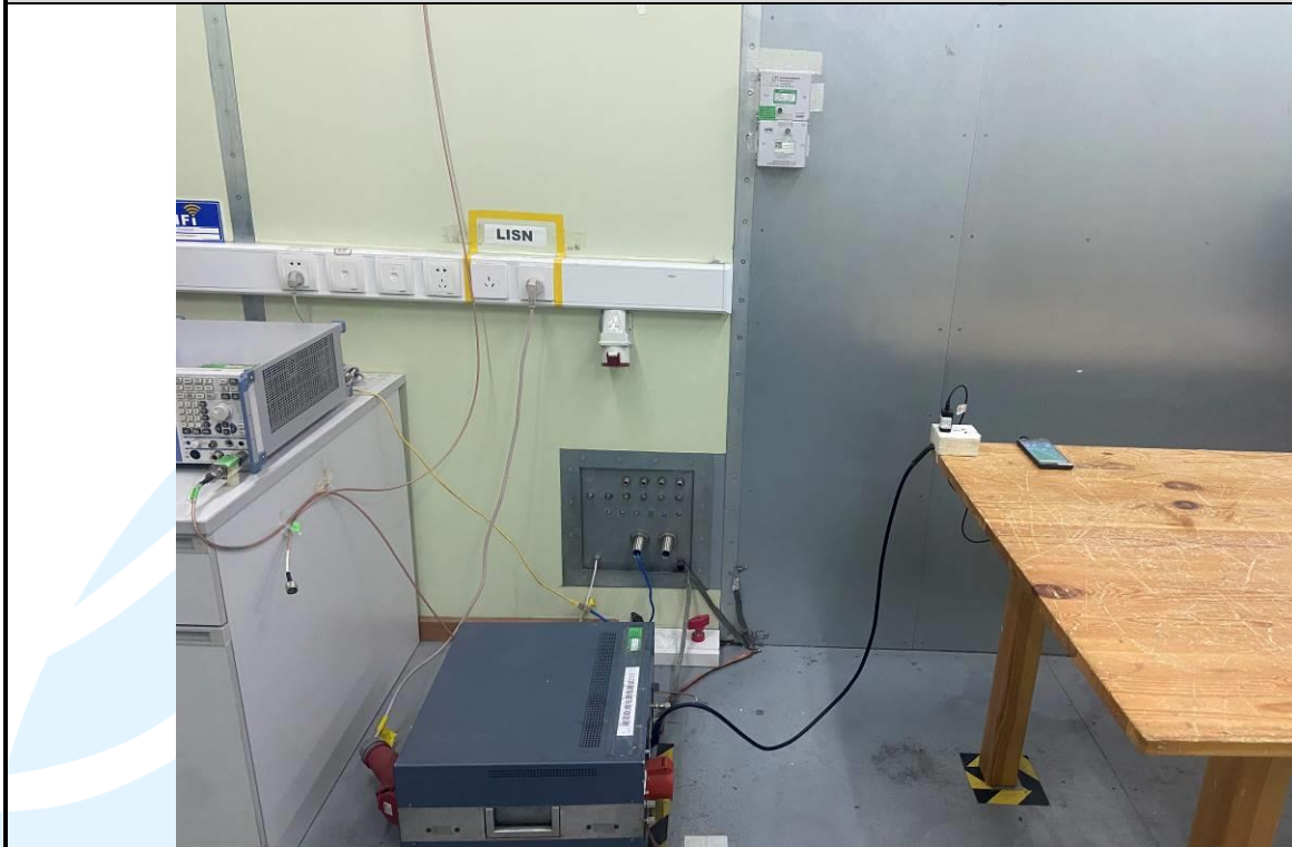
Conducted Emission Test Setup
