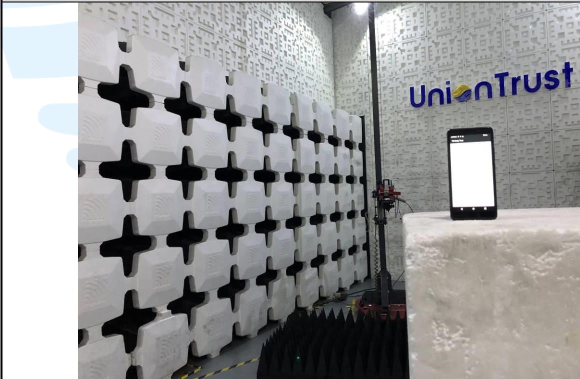
Radiated emission Test Setup (Above 1 GHz)
