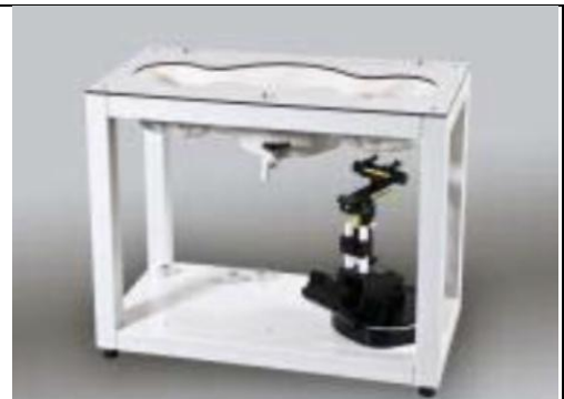
Fig. 6.8 Photo of SAM Phantom
