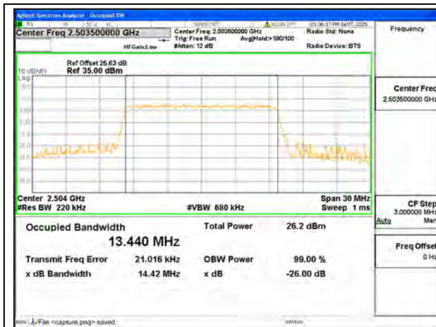
B41 / 15MHz / QPSK/ Low CH
