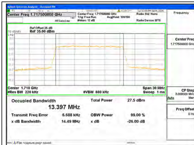
B4 / 15MHz / QPSK/ Low CH
