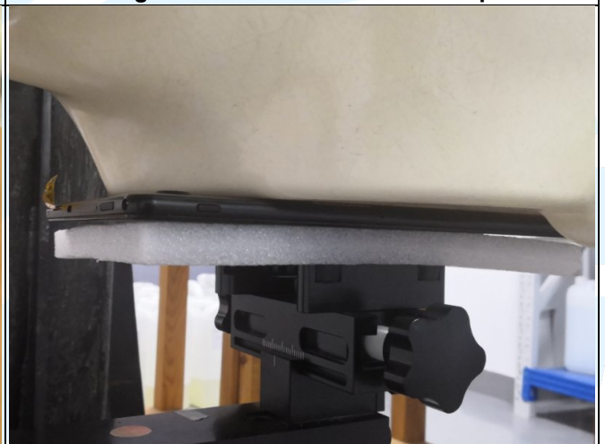
Rear Face of EUT with 0 cm Gap
