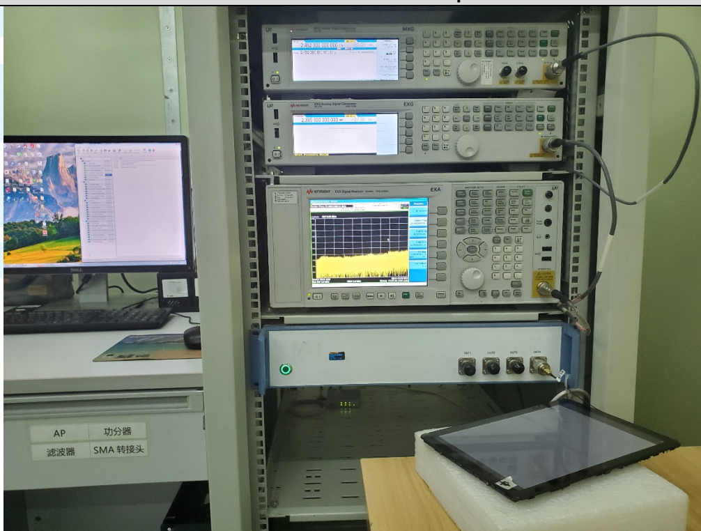
RF Conducted Test Setup
