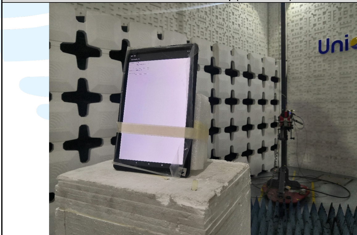
Radiated emission Test Setup (Above 1 GHz)
