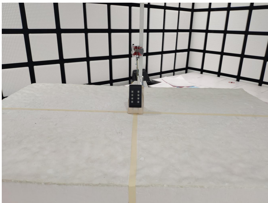
Radiated emission Test Setup-3 (above 1GHz)
