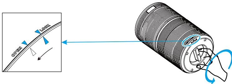
2. Remove the base cover and take out the new filter.
