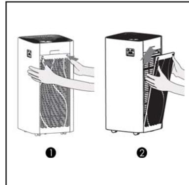
[3] Pull out the filter inside the purifier.
