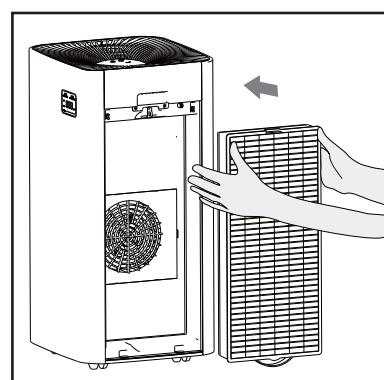
**[7]** Reinstall the filter cover, align and insert the fixed groove, and then press the button on the filter cover to apply pressure to secure the filter cover.
