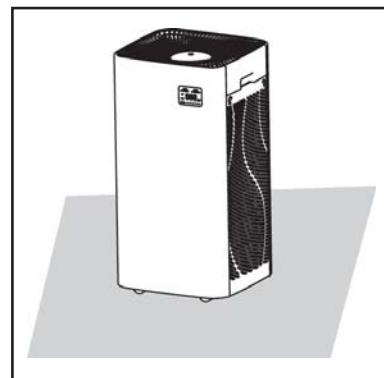
**[2]** Press the “
