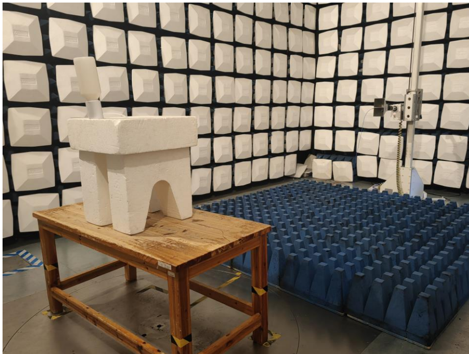
Test Setup For Radiated Emission (Above 1GHz)
