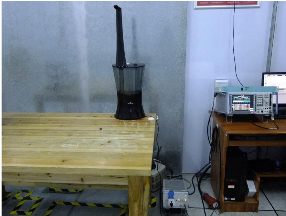
Test Setup For Conducted Emission
