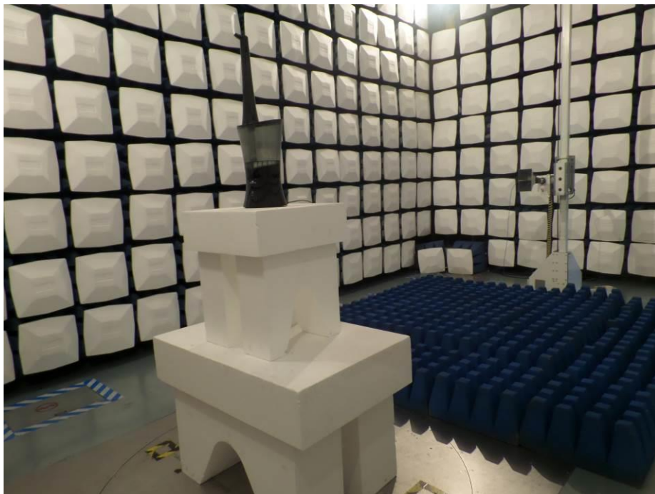
Test Setup For Radiated Emission (Above 1GHz)
