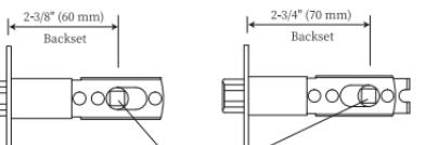
⚠ Mechanism will be horizontal. Note Curved edge of Handle Latch bolt should face in direction that door closes.
