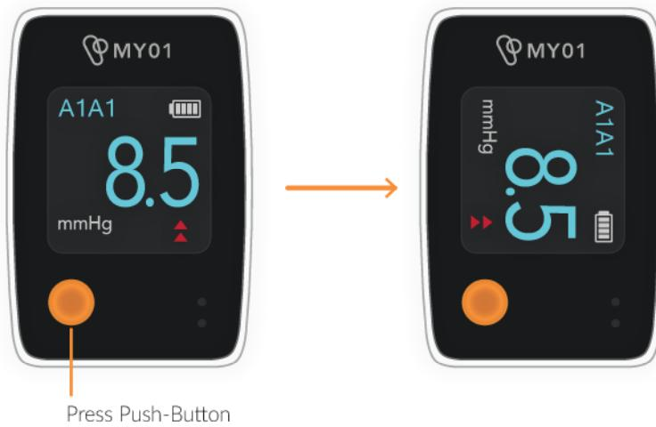
Figure 6 : Rotating Display Orientation
