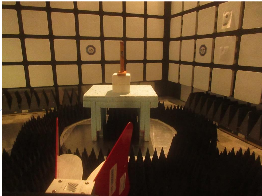
Photo 4: – Test Setup >1GHz – Horizontal Polarization
