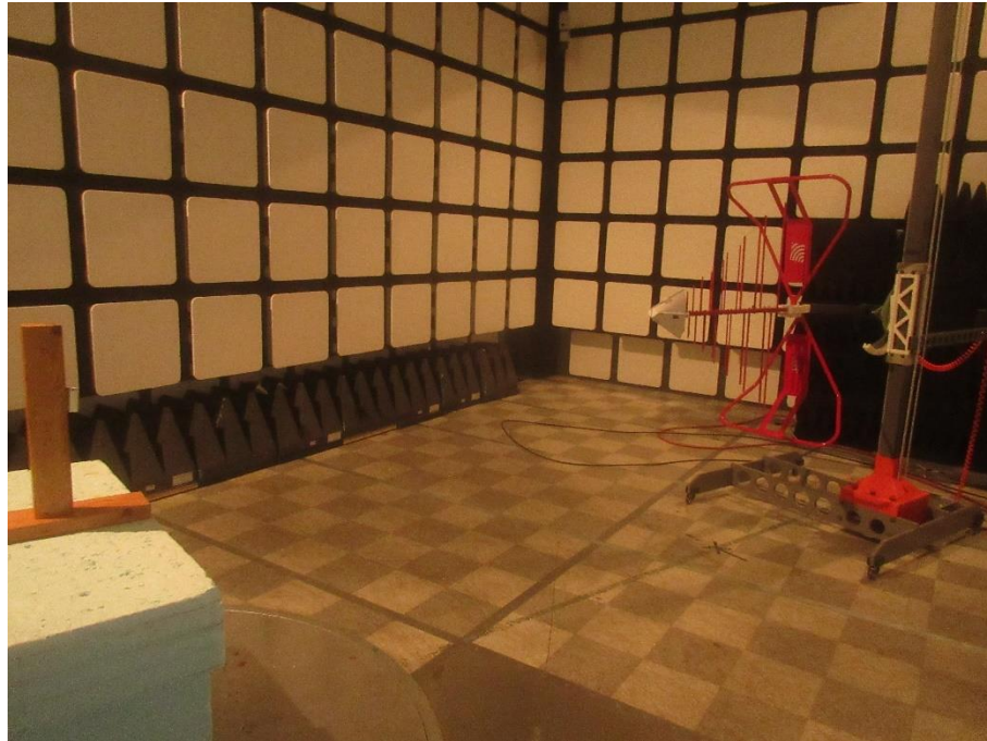
Photo 3: – Test Setup – 30MHz to 1GHz – Vertical Polarization
