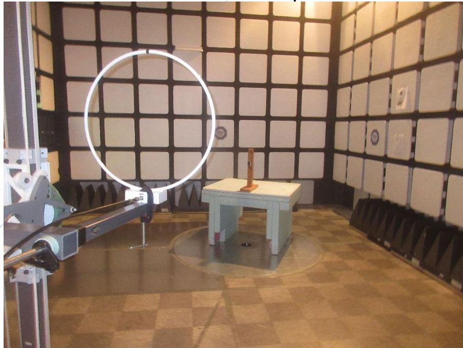
Photo 2: – Test Setup – 15kHz to 30MHz
