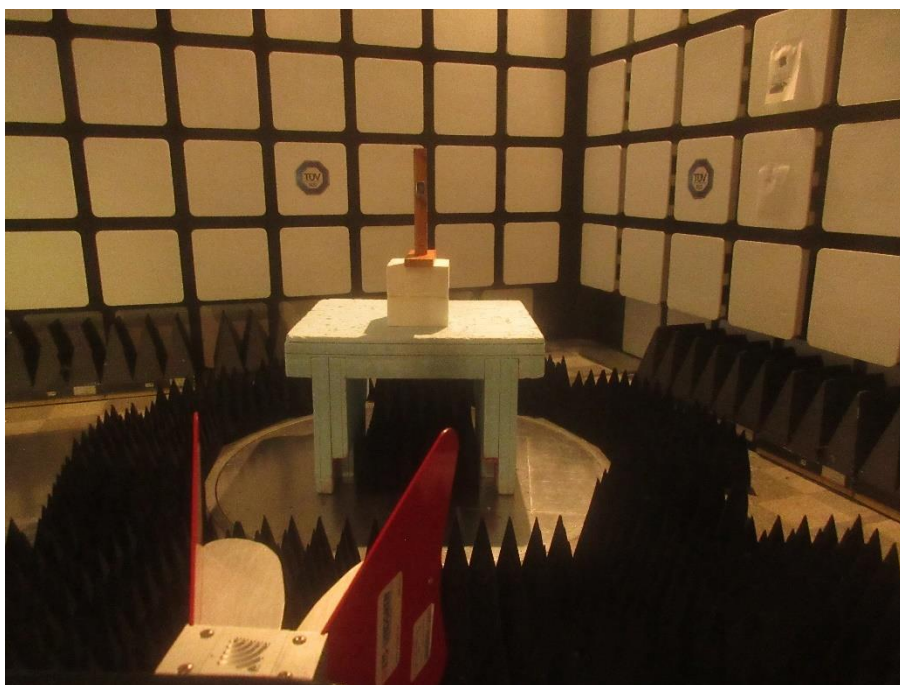
Photo 4: – Test Setup >1GHz – Horizontal Polarization
