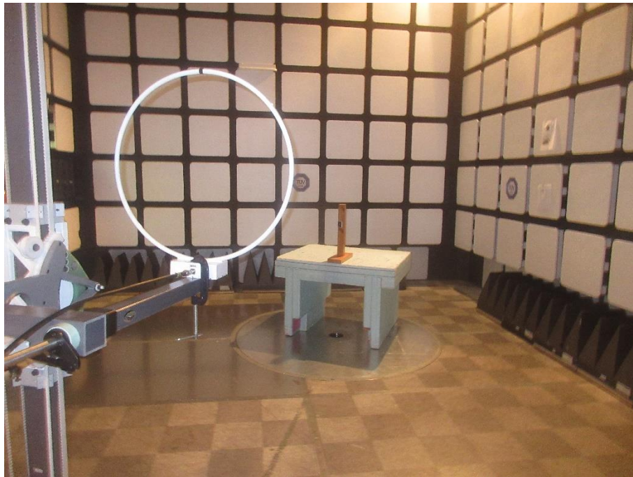
Photo 2: – Test Setup – 15kHz to 30MHz
