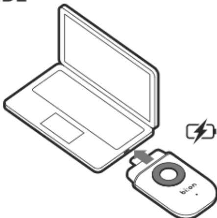
You can charge the device when you connect the charge with power supplies such as laptop, power bank or smartphone.
