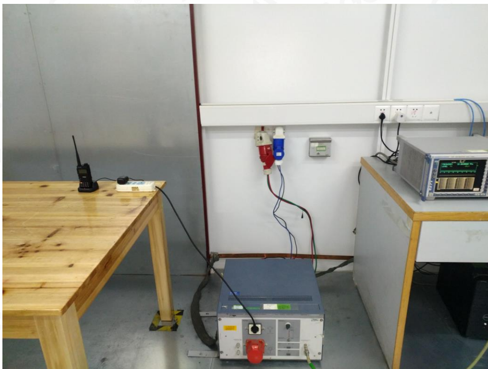
RADIATED EMISSION TEST SETUP-BELOW 1GHZ
