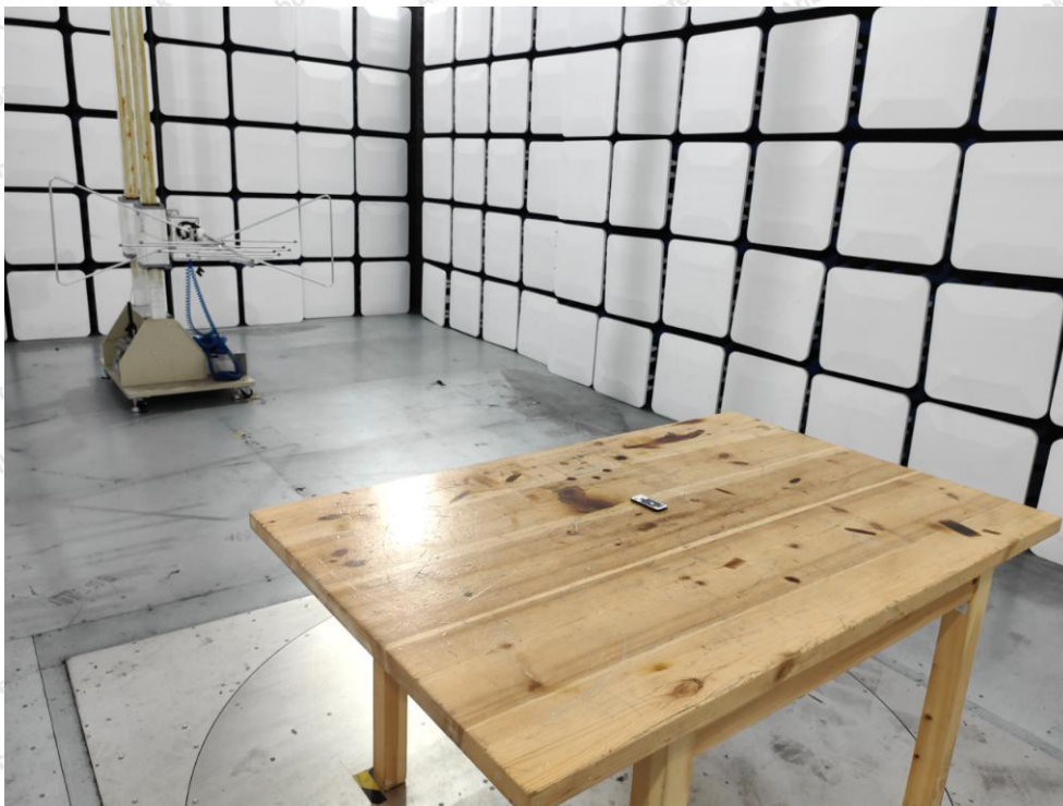
Photo of Radiated Emission Measurement
