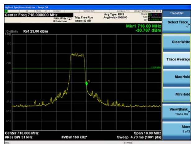
LTE Band 12 16QAM 3MHz CH-High, 1 RB
