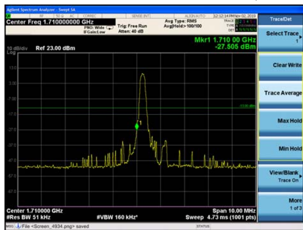
LTE Band 66 16QAM 1.4MHz CH-Low, 100%RB
