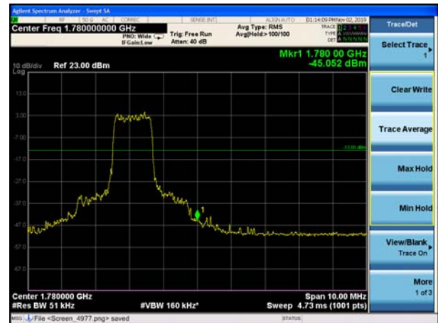
LTE Band 66 16QAM 1.4MHz CH-High, 1 RB
