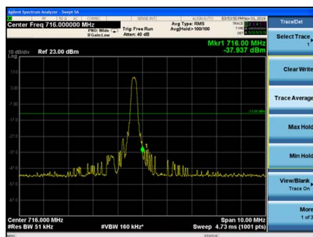
LTE Band 12 16QAM 5MHz CH-High, 100%RB
