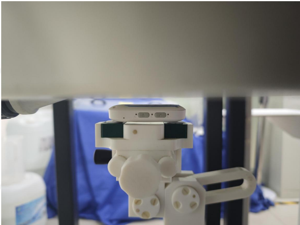
Body Back side(separation distance is 10mm)
