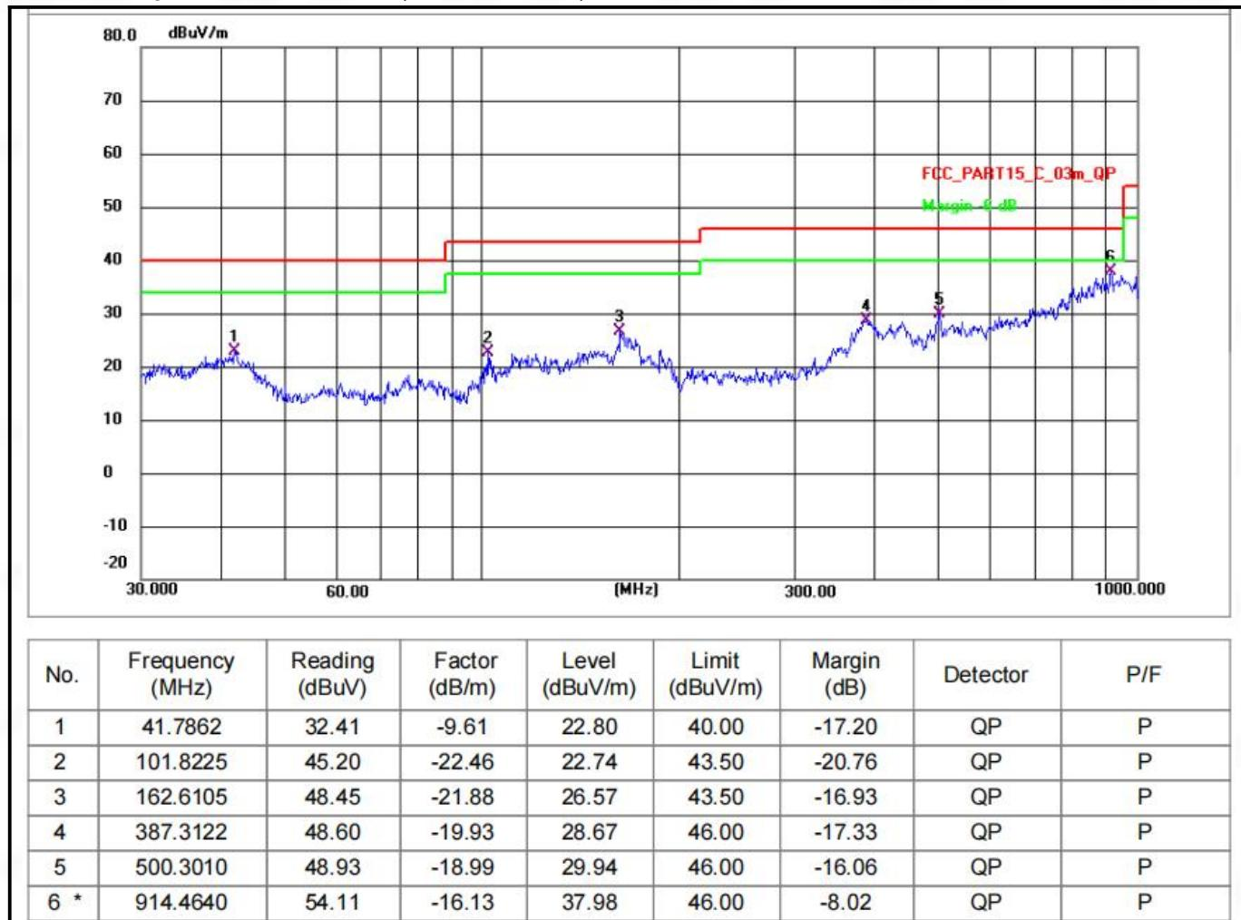
Note1:Level=Read Level + Antenna Factor + Cable Loss - Preamp Factor
