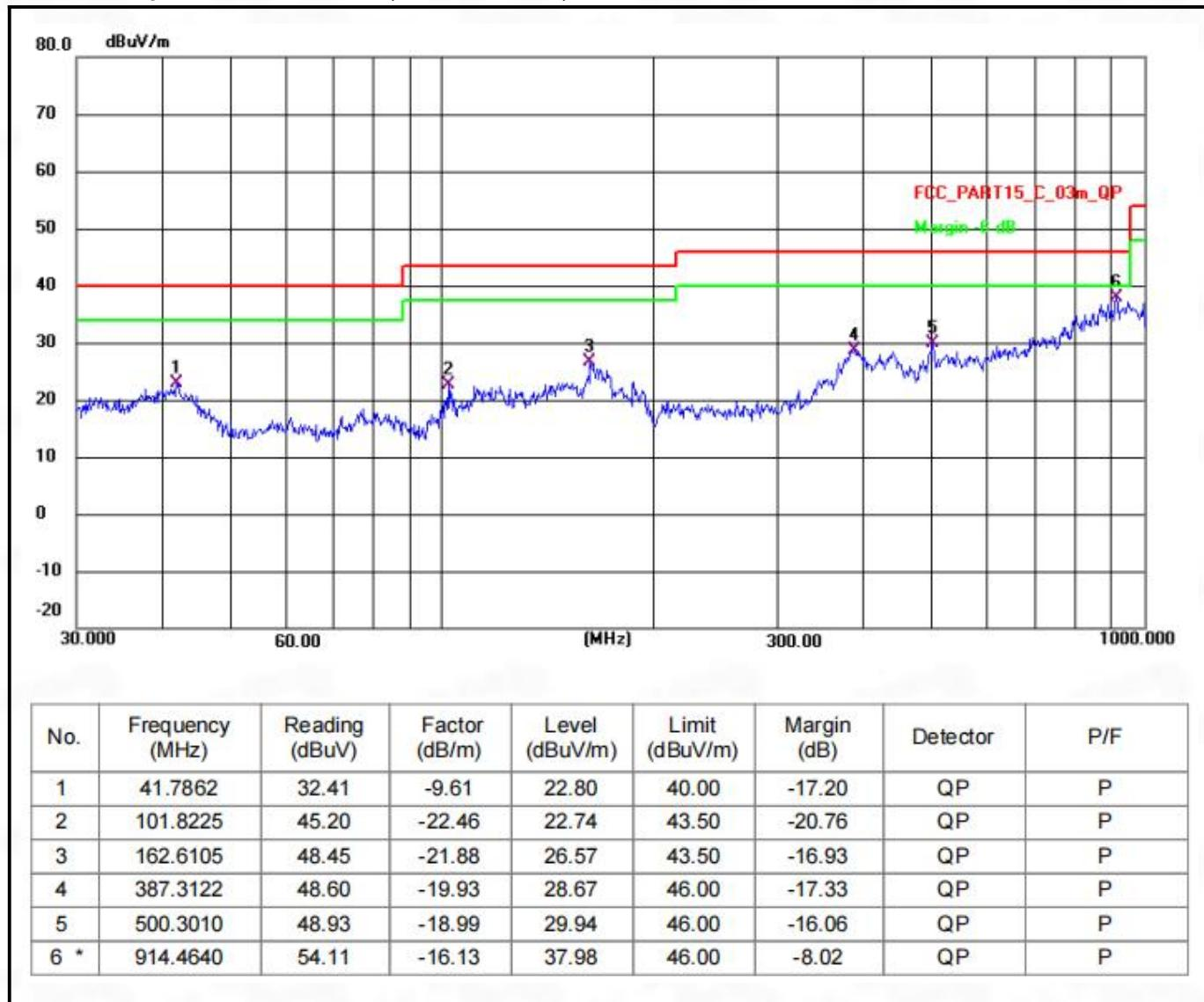
Note1:Level=Read Level + Antenna Factor + Cable Loss - Preamp Factor
