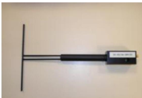
Figure 1 – Satimo COMOSAR Validation Dipole
