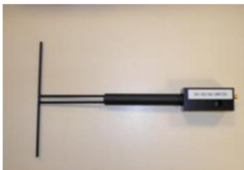
Figure 1 – Satimo COMOSAR Validation Dipole
