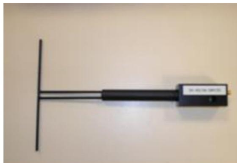
Figure 1 – Satimo COMOSAR Validation Dipole
