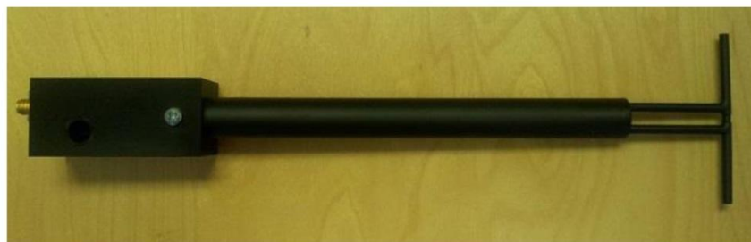
Figure 1 – MVG COMOSAR Validation Dipole
