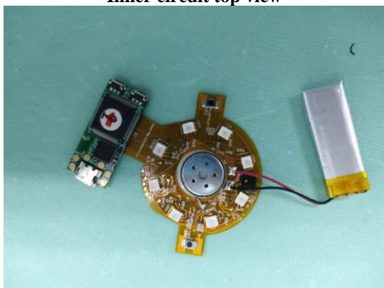
Inner circuit top view
