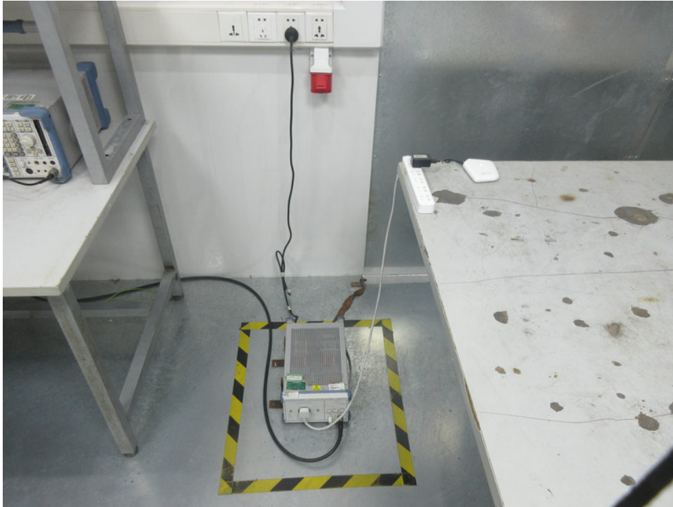
Photo of Conducted Emission Measurement
