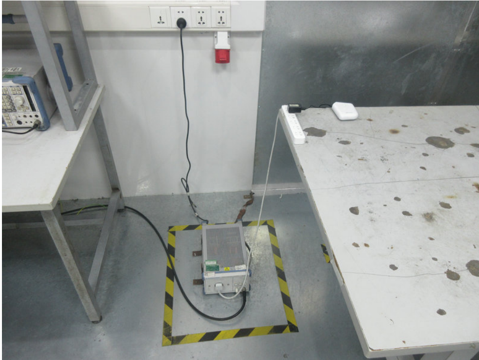
Photo of Conducted Emission Measurement
