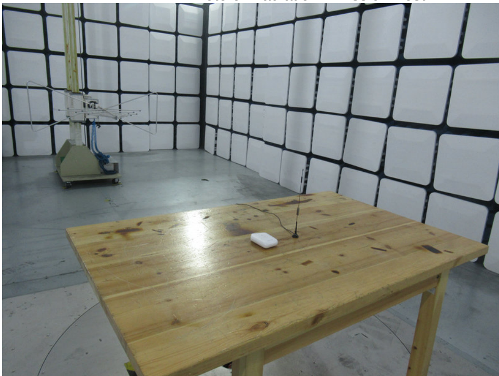
Photo of Radiation Emission Test
