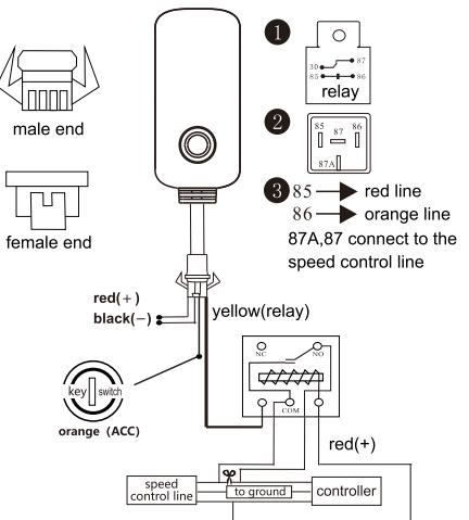
① Red line connect battery positive pole(+) black line connect battery negative pole(-).
