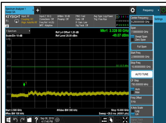
GFSK,2480MHz,DH5,Plot 1,Band Edge
