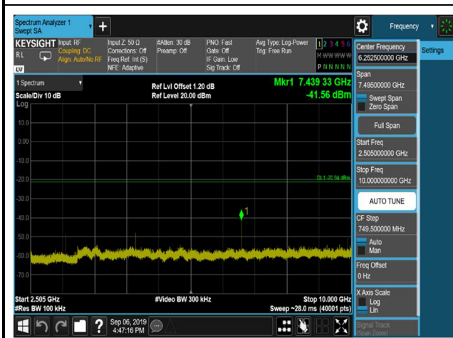
8DPSK,2480MHz,3DH5,Plot 3,2505MHz~100 00MHz
