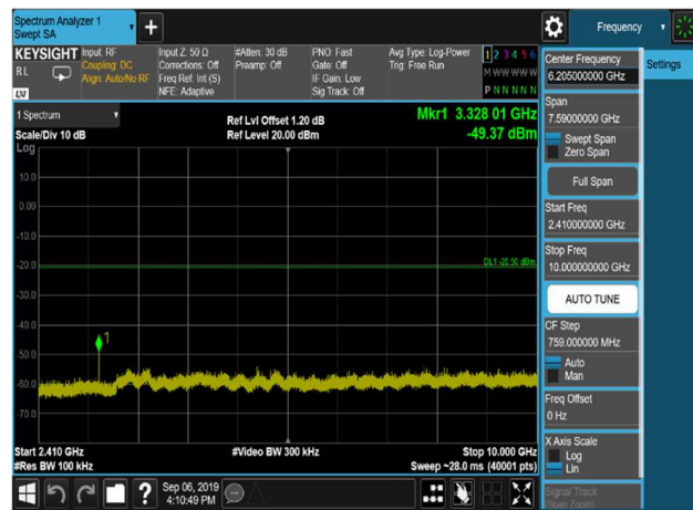
GFSK,2441MHz,DH5,Plot 1,Band Edge
