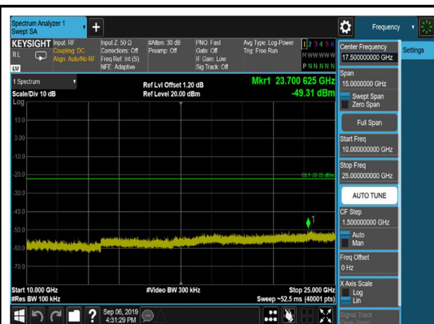
DQPSK,2480MHz,2DH5,Plot 2,0.009MHz~24 75MHz
