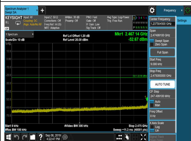
GFSK,2480MHz,DH5,Plot 4,10000MHz~2500 0MHz
