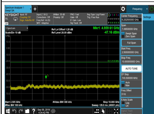
8DPSK,2402MHz,3DH5,Plot 1,Band Edge
