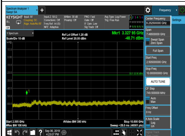
DQPSK,2402MHz,2DH5,Plot 1,Band Edge
