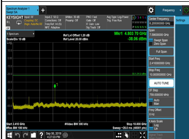
DQPSK,2441MHz,2DH5,Plot 1,Band Edge
