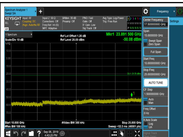
8DPSK,2480MHz,3DH5,Plot 2,0.009MHz~24 75MHz
