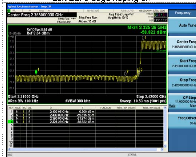
Left Band edge hopping on
