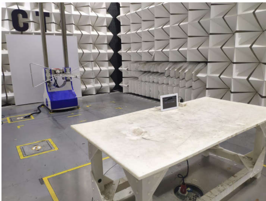
Radiated spurious emission Test Setup-2(Below 1GHz)
