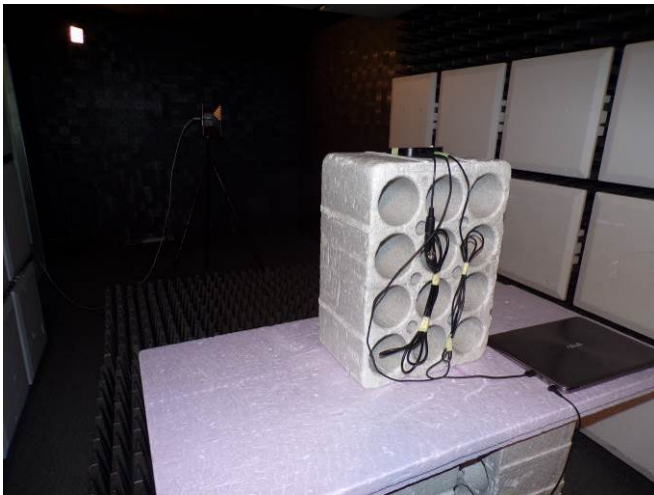
FAC setup (1GHz-25GHz / 3m)
