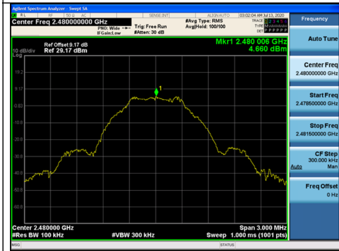
GFSK on Channel 39
