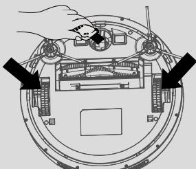
Clean the wheels in front and on both sides of the machine with the cleaning brush regularly.
