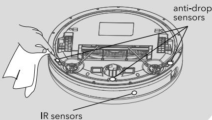
It is suggested to clean the sensors with dry cloth carefully after each time cleaning. It will avoid the dust store on sensors to affect the performance of the machine.
