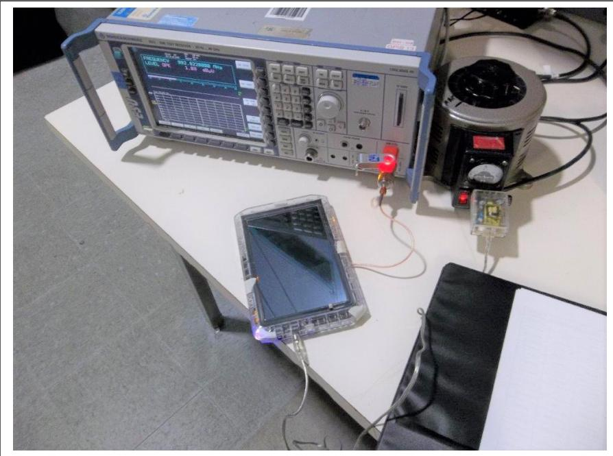
**Radiated Spurious Emissions, Less Than 30 MHz**
