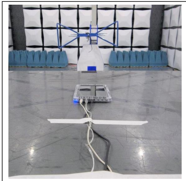
**Radiated Spurious Emission, above 1 GHz**
