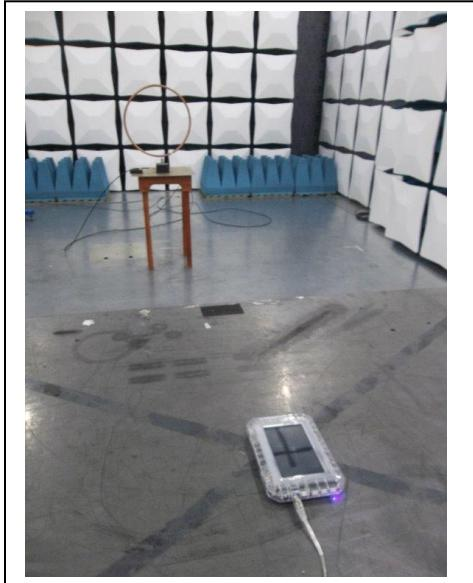
**Radiated Spurious Emission, 30 MHz to 1000 MHz**
