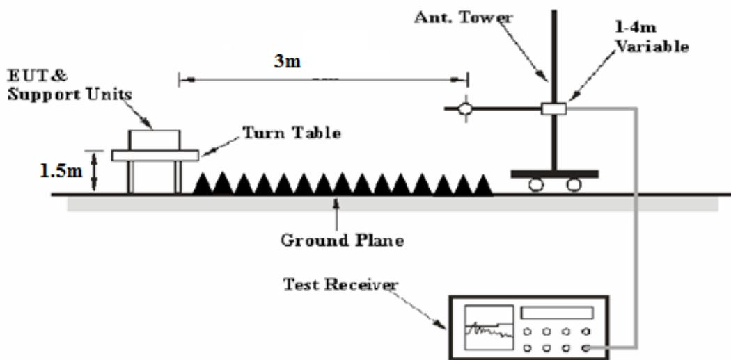
The radiated emission below 1GHz tests were performed in the 3 meters chamber test site A, above 1GHz tests were performed in the 3 meters chamber test site B, using the setup accordance with the ANSI C63.10-2013. The specification used was the FCC 15.209, and FCC 15.249 limits and the RSS-Gen, and RSS-210 limits.
