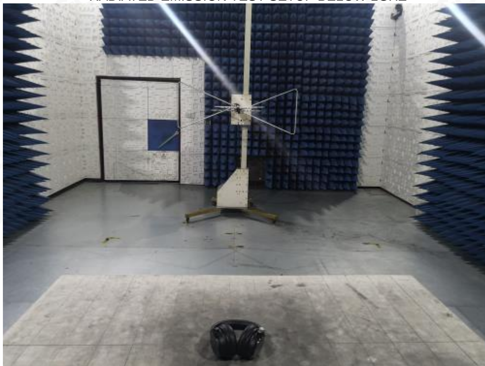
RADIATED EMISSION TEST SETUP BELOW 1GHZ
