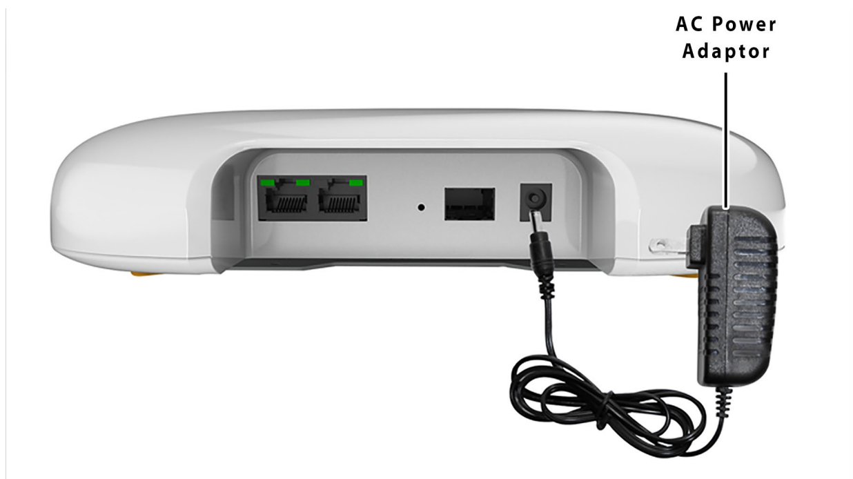
Figure 12: Power up the device using AC Adaptor (12V)
