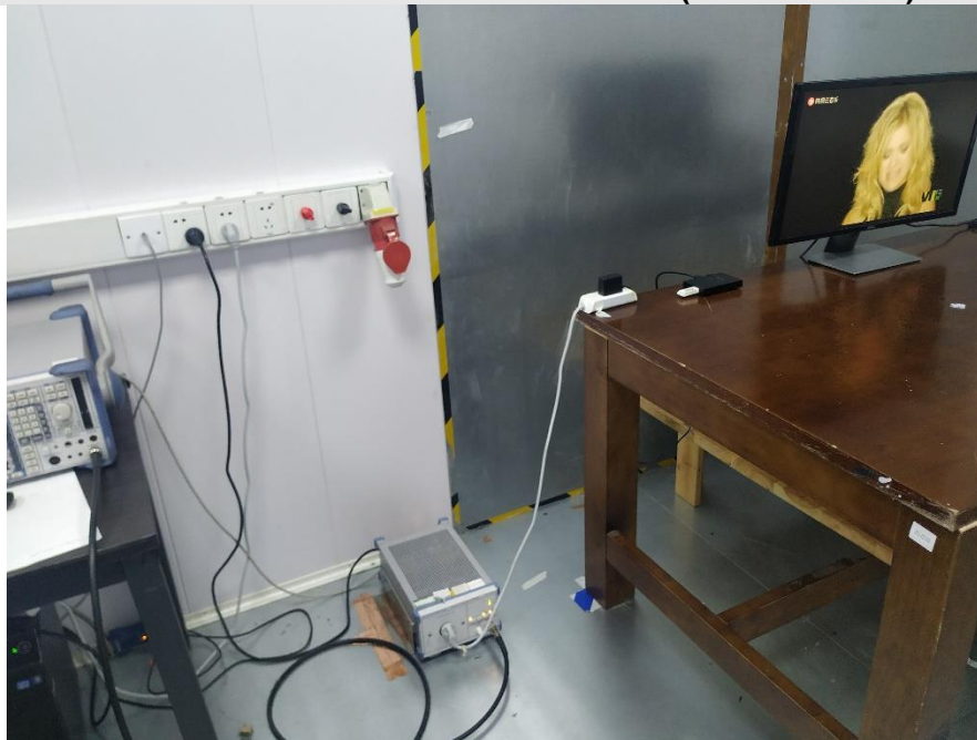
Conducted Emissions at AC Power Line (150kHz-30MHz)
