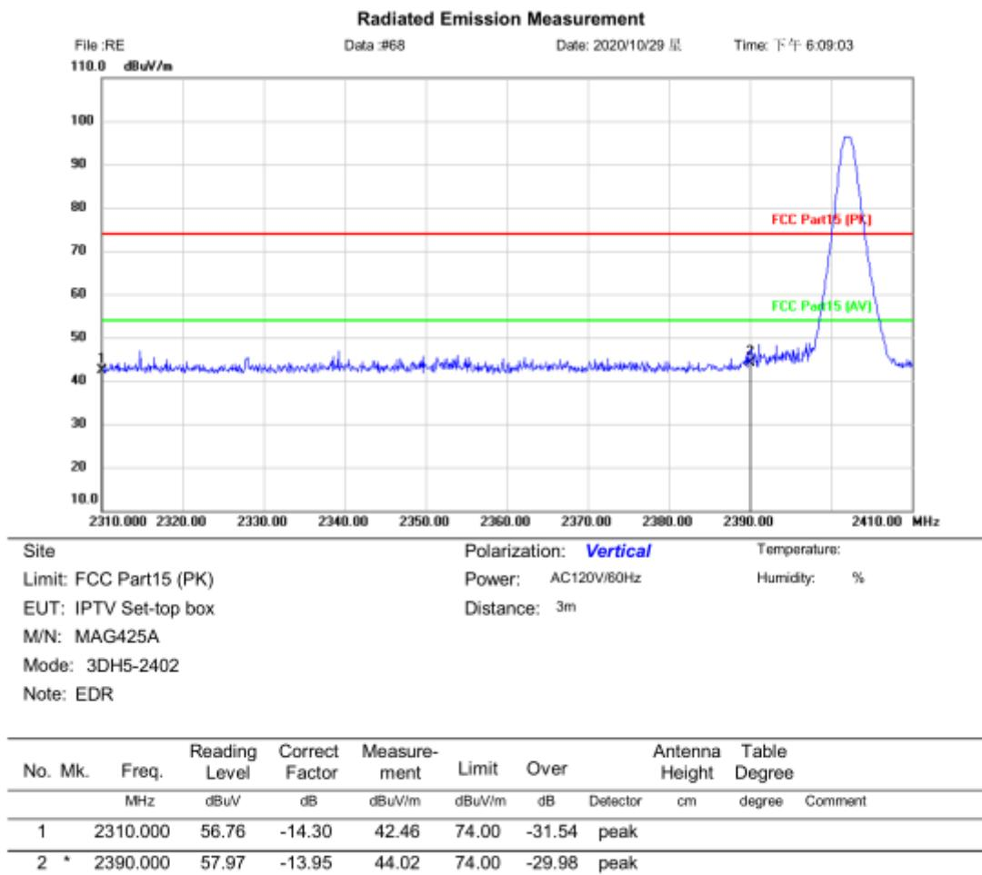
**Radiated Emission Measurement**
