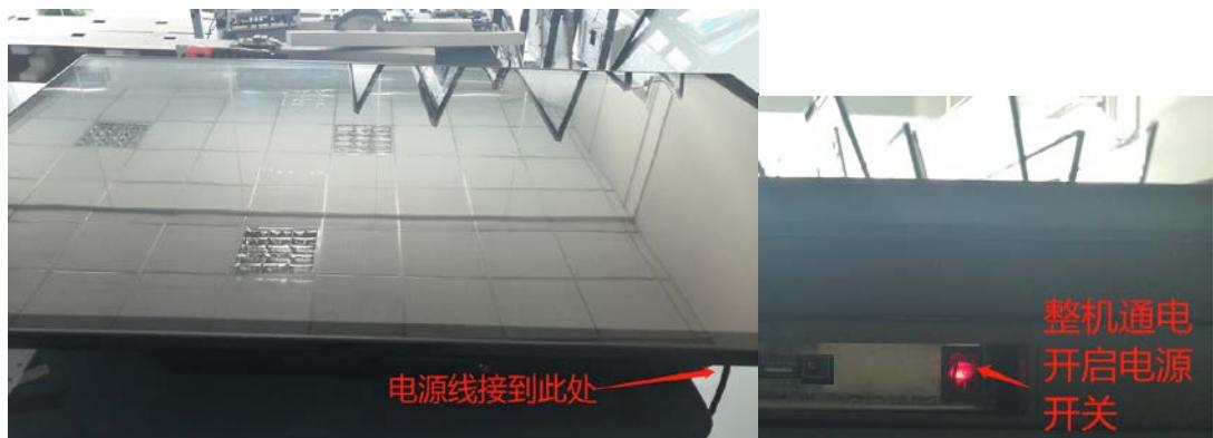
电源线接到此处 Power supply wire connect to here 整机通电 One machine power
