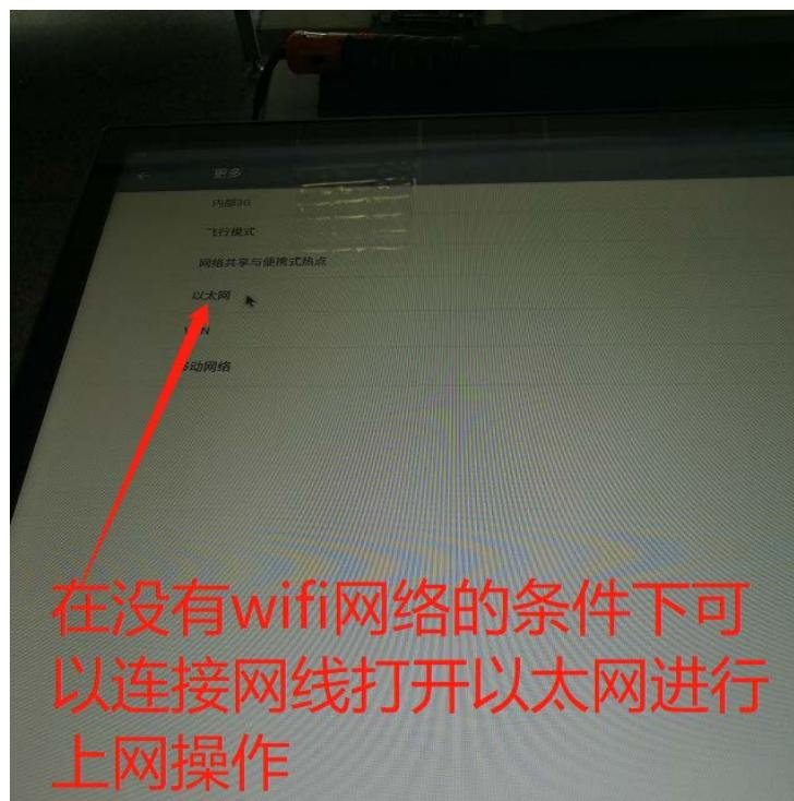
在没有 WiFi 网络的条件下可以连接网线打开以太网进行上网操作 Can connect network wire open Ethernet network to online operating under the condition that no WiFi network
