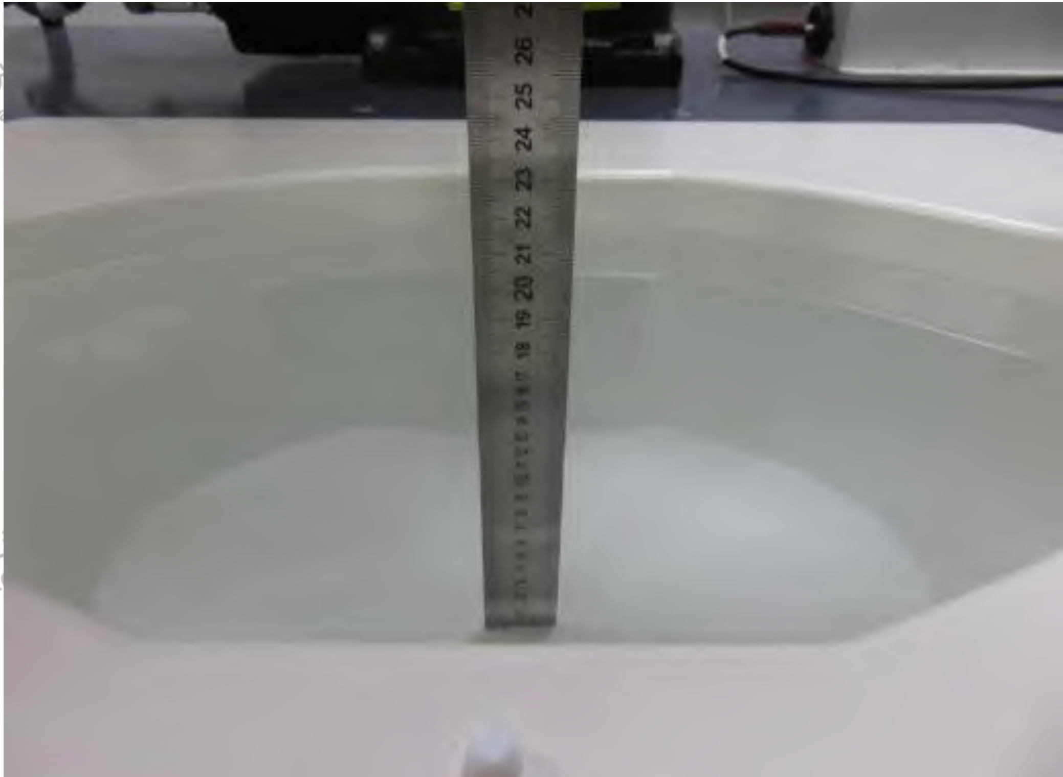
Photograph of the depth in the Body Phantom (5800MHz, 15.4cm depth)
