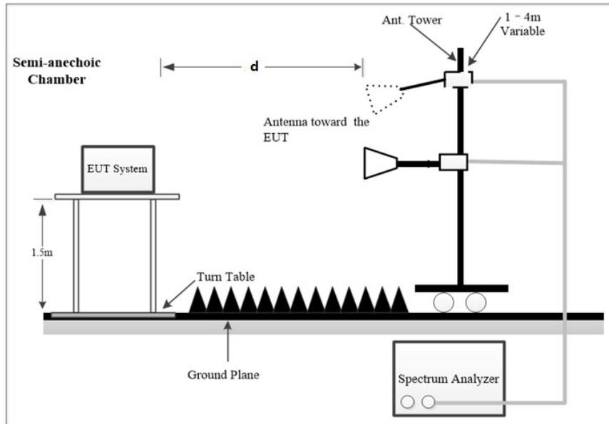
The radiated emission tests using the setup accordance with the ANSI C63.10-2020. The specification used was the FCC 15.209, FCC 15.247, RSS-247, RSS-Gen limits.
