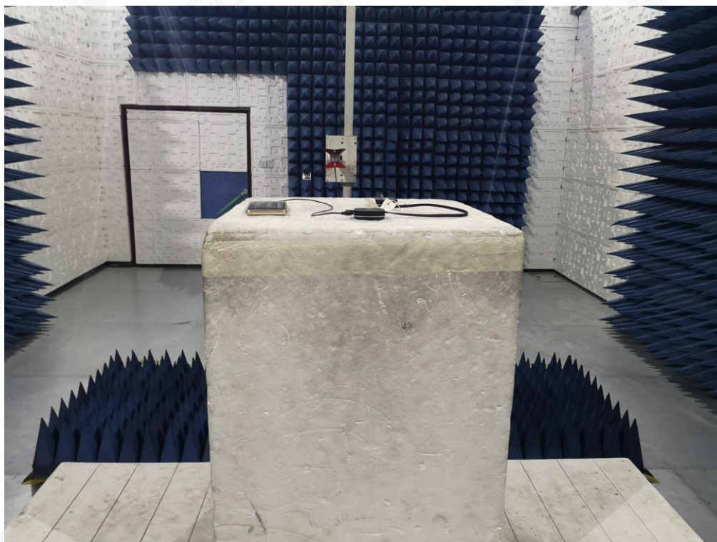
RADIATED EMISSION TEST SETUP ABOVE 1GHZ
