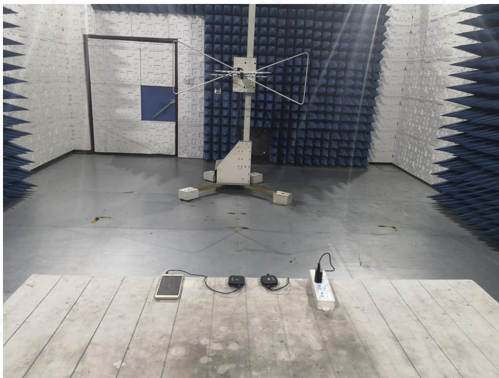
RADIATED EMISSION TEST SETUP ABOVE 1GHZ
