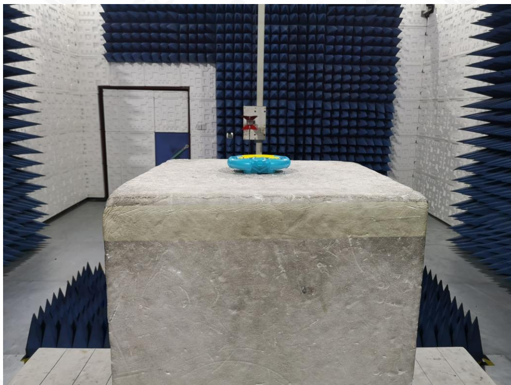
FCC RADIATED EMISSION TEST SETUP ABOVE 1GHZ
