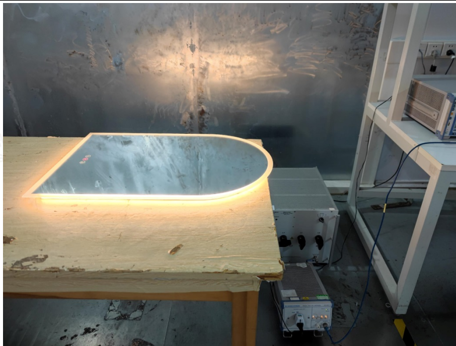
Conducted emissions on AC mains
