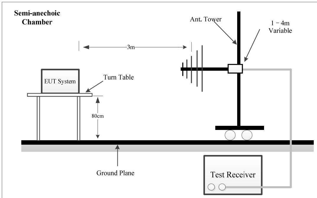
The radiated emission tests were performed at the 3 meters distance, using the setup accordance with the ANSI C63.4-2014. The specification used was the FCC Part 15B Class B limits.
